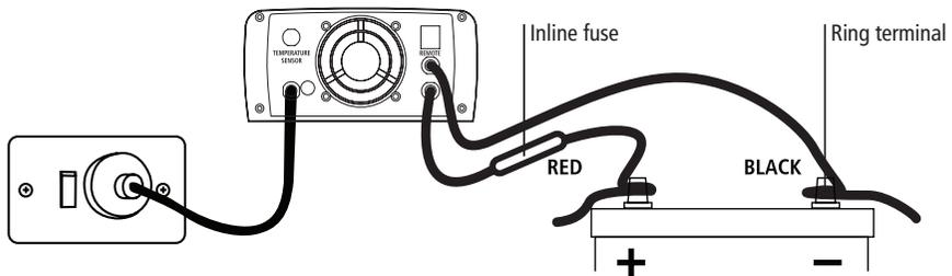
If the charger is used in a Permanent/Hard Wired application and the vehicle will not be used for some time, it is best to leave the charger connected to mains power (turned 'On') so that it can maintain the battery fully charged.
