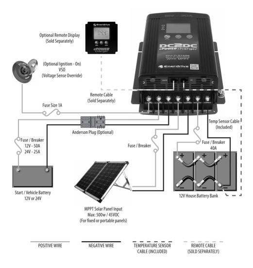
This diagram is for a referance only. No cables, fuse/breakers, batteries or solar panels are supplied with this unit.
